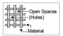
Mesh as a measurement describes more generally aperture opening (space between wires and wire material) expressed in the number of wires needed to create these openings.
